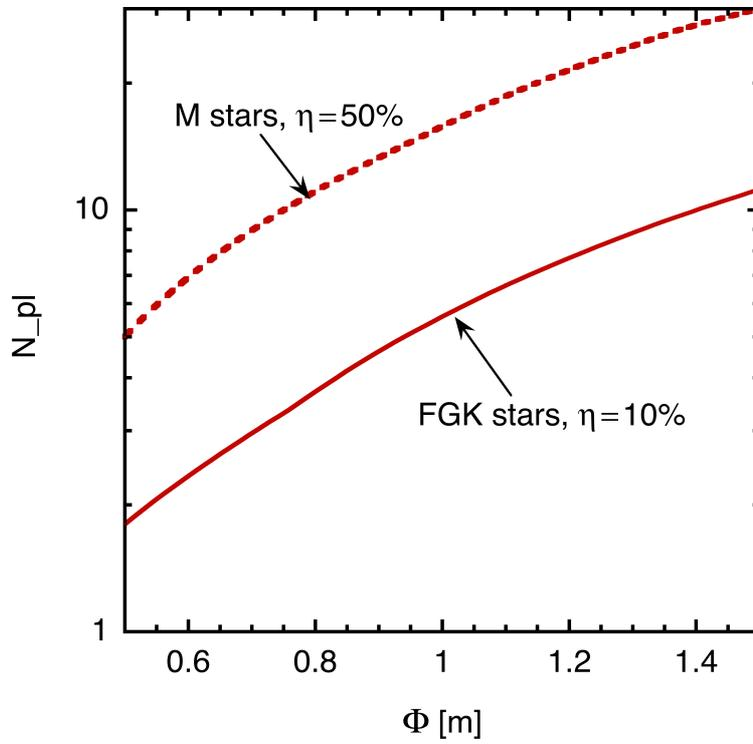
*Figure 2: the number of planets that can be studied by an interferometer around FGK and M stars, as a function of the diameter of the four collecting mirrors, for a spectral resolution  $\lambda/\Delta\lambda = 20$  (spectroscopy),  $1.5 R_{earth}$  planets located at  $1.3 L^{1/2}$  [AU], and a prior identification of the suitable stars. The mission is 5 yr long, 1 yr is spent on M stars with  $\eta_{earth\_M} = 50\%$ , 4 yrs are spent on FGK stars with  $\eta_{earth\_FGK} = 10\%$ .*
